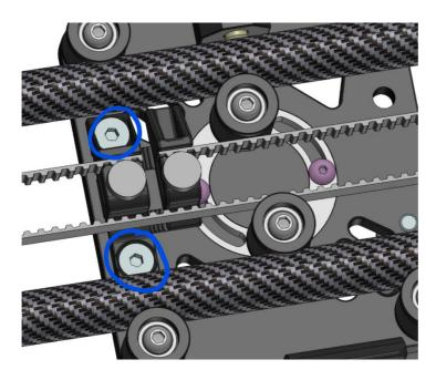
2. Push the right clamp together until the desired toothed belt tension is achieved and tighten the countersunk screws again (max. 2.5Nm).
