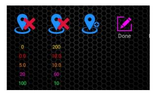
All position values and frame numbers can now be changed manually by tapping on the values. A dialog box will appear in which you can adjust values. You can also move individual motors to the selected keyframe positions.
