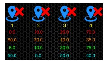
All position values can now be changed manually by tapping on the values. A dialog box will appear in which you can adjust values. You can also move individual motors to the selected keyframe positions.
