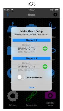
Once all profiles are selected, tap the "Done" button to exit the Quick Setup. All settings will now be transferred to the PINE Controller.
