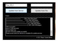
V. At the end of the update process, the PINE Controller needs to be restarted by disconnecting and reconnecting the power supply.
