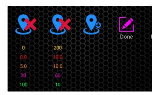
All position values and image numbers can now be changed manually by tapping on the values. A dialog box will appear where you can adjust values. You can also move individual motors to the selected keyframe positions.
