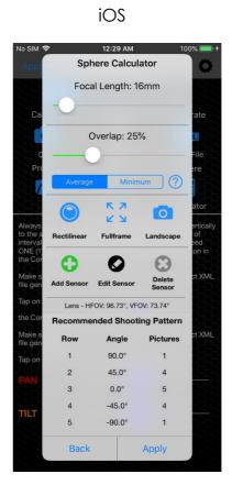
Within the sphere calculator, you can make various settings regarding your camera equipment (focal length, sensor, etc.). In the lower part of the dialog you will be given recommendations about the number of vertical rows and horizontal columns. The recommendations can be accepted directly via the "Apply" field and you do not have to make any further settings for the rows and columns.
