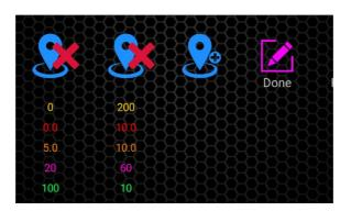
All position values can now be changed manually by tapping on the values. A dialog box will appear in which you can adjust values. You can also move individual motors to the selected keyframe positions.
