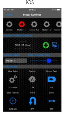
The **motor profiles** can also be set under the motor settings (similar to the Motor Quick Setup). Further profiles can also be added via the Motor Setup Wizard. To do this, click on the green **a** symbol.
